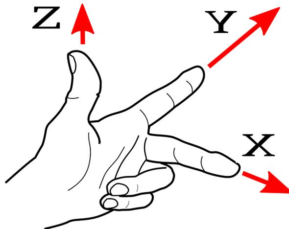
Mount your stepper motors into your CNC, if you haven't already done so. Send Grbl some motion commands, such as `G91 G0 X1` or `G91 G0 X-1`, which will move the x-axis +1mm and -1mm, respectively. Check all axes. If an axis is not moving correctly, alter the `$3` direction port mask setting to invert the direction.
