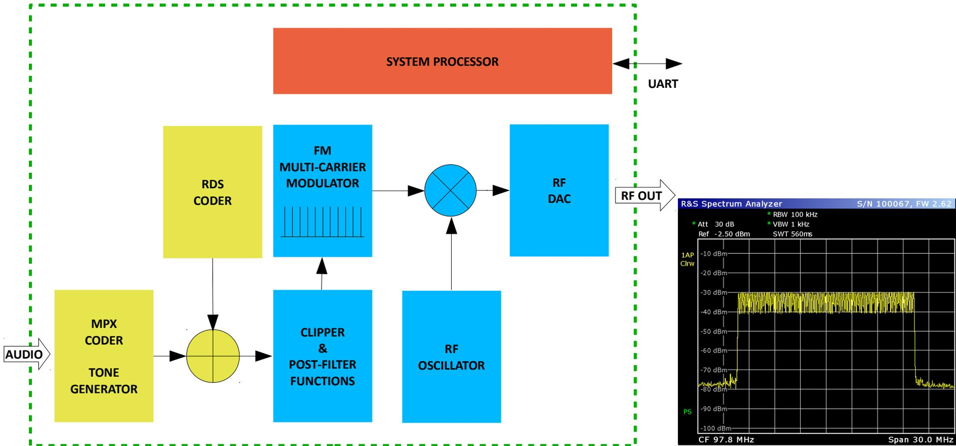
Special application for emergency alerts: the system transmits an alert tone or an audio and RDS message on all FM channels simultaneously. For example, it can transmit an alert message about an approaching ambulance or train, or a warning message in case of a problem in a road tunnel. The module uses the RDS Traffic Alert to automatically switch from CD/MP3 player to FM Radio.
